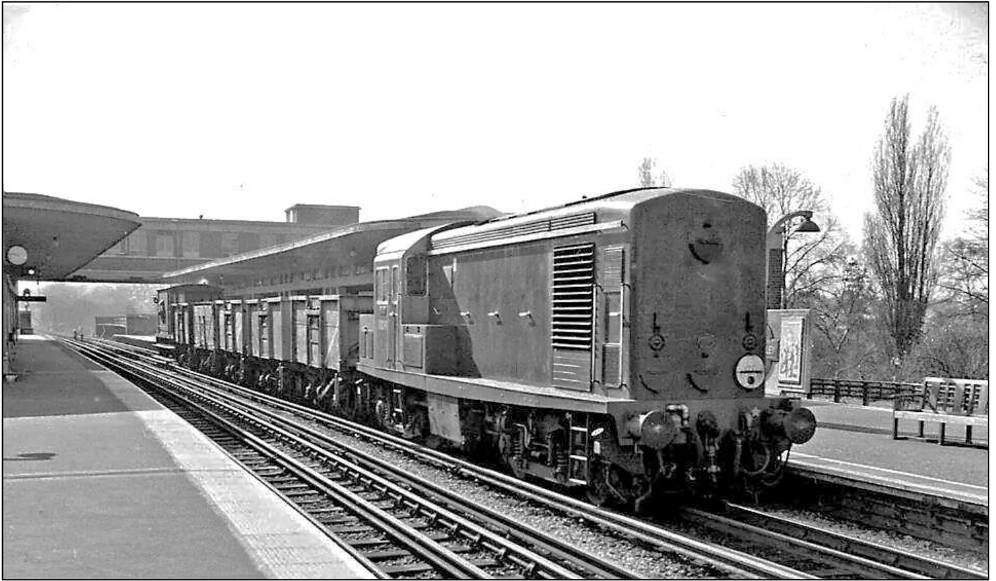
Above: One of the class 15 Bo-Bo diesel locos trundles north through East Finchley middle platform 2 in the closing days of freight trains on the Northern Line.
